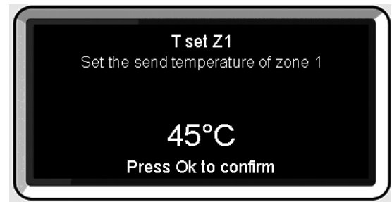
Change heating hot water temperature
